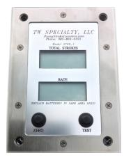
Model 5700-1 monitors up to 1 pump and displays total strokes and rate per minute for the pump. The test button will test the unit @ 60 SPM. Zero buttons are used to zero total strokes.
