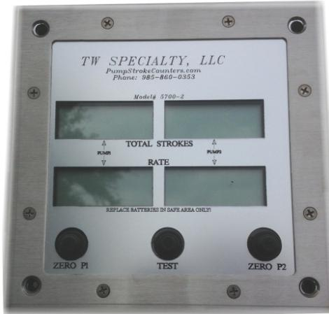
Model 5700-2 monitors up to 2 pumps and displays total strokes and rate per minute for the pump. The test button will test the unit @ 60 SPM. Zero buttons are used to zero total strokes.
